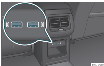
Fig. 195 Rear part of the centre console: USB connectors.
