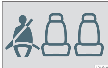
Fig. 4 Instrument panel: left rear seat occupied and corresponding seat belt fastened display.
