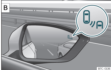
Fig. 225 In the exterior mirrors: blind spot detector indication.
