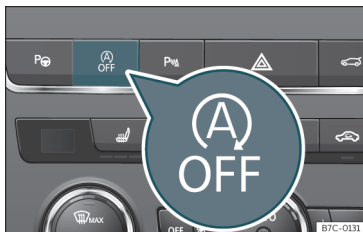
Fig. 199 Centre console: Start-stop system button.
