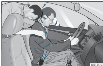
Fig. 7 The unbelted passenger in the rear seat is thrown forward violently, hitting the driver who is wearing a seat belt.
