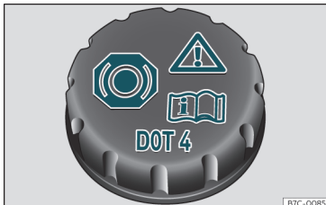
Fig. 261 Engine compartment: brake fluid reservoir cap.
