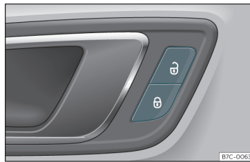
Fig. 70 Driver's door: central locking switch.
