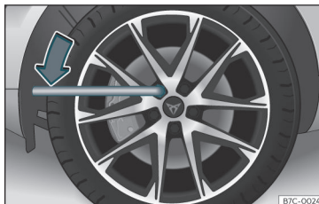
Fig. 32 Wheel change: loosen the wheel nuts.
