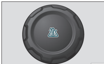
Fig. 260 Engine compartment: coolant expansion tank cap.
