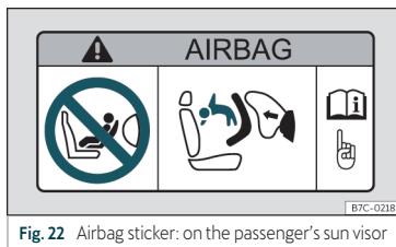
Fig. 22 Airbag sticker: on the passenger's sun visor
