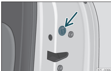
Fig. 75 Locking the door manually.
