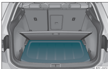
Fig. 107 In the luggage compartment: fitting the rear shelf.
