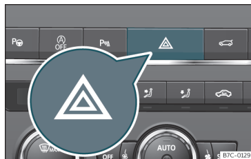
Fig. 90 Dash panel: hazard warning lights switch
