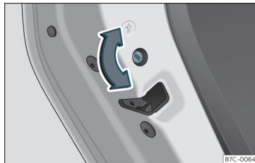
Fig. 76 Childproof lock on the left hand side door.
