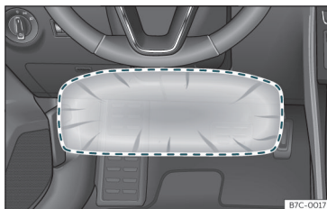
Fig. 17 On the driver side: airbag action radius for the knees.
