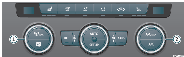
Fig. 122 In the centre console: Climatronic controls.
