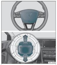
Fig. 12 Driver airbag located in steering wheel.
