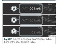
The speed limiter helps avoid exceeding a programmed speed, from 30 km/h (19 mph) approx. and faster. >>>  $\Delta$
