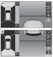
Fig. 246 Display on the top view system screen: A Front camera: off-road view. B Rear camera: off-road view.
