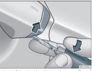
Fig. 74 Driver door handle: lever the cover off
