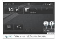
$\mathsf{MirrorLink}^{\circledast}$  is a protocol which enables communication between a device and the Infotainment system.
