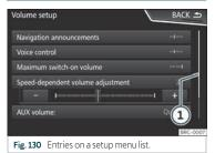
The entries on a list can be activated by pressing them on the screen or by using the settings button.
