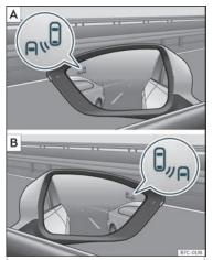
Fig. 225 In the exterior mirrors: blind spot detector indication.
