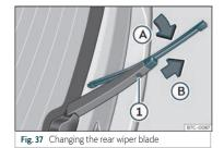
The windscreen wiper blades are supplied as standard with a layer of graphite. This layer is responsible for ensuring that the wipe is silent. If the graphite layer is damaged, the noise of the water as it is wiped across the windscreen will be louder.
