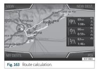
When starting route guidance, the route is calculated based on the data that have been selected in the **Route options** menu.
