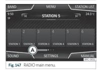
In the *Radio* main menu, you can store stations from all available frequency wavelengths on the numbered function buttons. These function buttons are called "memory buttons".
