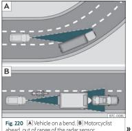
ahead, out of range of the radar sensor.
