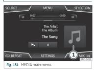
The tracks of the Media source that is being listened to can be changed successively using the arrow buttons.
