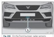
A radar sensor is installed on the front bumper to determine the traffic situation **339** Fig. 216 (1).
