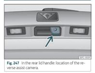
A camera installed in the rear lid handle assists the driver with reverse parking or manoeuvring **>>> Fig. 247**.
