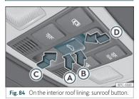
The sun blind automatically opens along with the sunroof if completely closed or if in front of the sunroof. The sun blind remains in the previous position and does not automatically close with the sunroof. The sun blind can only be closed completely once the sunroof has been closed.
