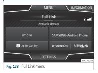
When you enter Full Link for the first time, the technologies available for pairing the portable device are displayed.
