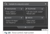
Many of the radio, media, telephone and navigation functions can be changed by voice commands.
