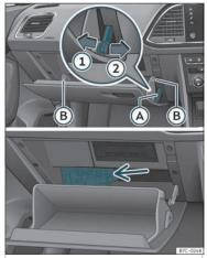
Fig. 44 Glove box (right hand drive): fuse box access.
