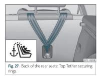
Child seats with the Top Tether system come with a strap for securing the seat to the vehicle anchor point, located at the back of the rear seat backrest and provide greater restraint.
