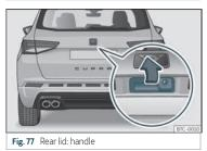
The rear lid opening system operates electrically. It is activated by exerting slight pressure on the handle **>>> Fig. 77**.
