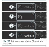
The cruise control system (CCS) is able to maintain the set speed from 20 km/h (15 mph).
