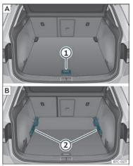
Fig. 108 Variable luggage compartment floor: A raised position; B lowered position.
