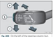
Fig. 209 On the left of the steering column: but tons to operate the speed limiter.
