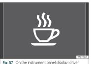
Fig. 57 On the instrument panel display: driver alert system symbol.
