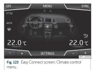
In the Easy Connect system it is also possible to perform various adjustments to the Climatronic.
