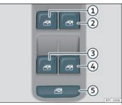
Fig. 83 Detail of the driver's door: window controls.
