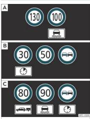
Fig. 58 On the instrument panel display: examples of speed limits or overtaking prohibitions with their respective additional signs.
