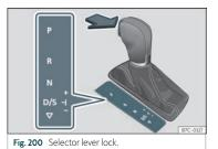
The selector lever position is shown when the corresponding sign lights up. With the selector lever in the manual gearbox positions **M**, **D** and **S**, the engaged gear is also shown on the display.
