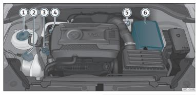
From time to time, the levels of the different fluids in the vehicle must be checked. Never fill with incorrect fluids, otherwise serious damage to the engine may be caused.
