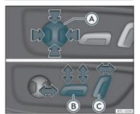
Fig. 97 Driver's seat: electric seat settings.
