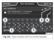
The on-screen keypad is used for functions such as entering an memory name, selecting
