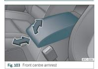
To *lift* the central armrest, lift it upwards in the direction of the arrow **>>> Fig. 103**, setting by setting.
