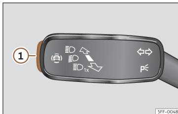
Fig. 57 On the turn signal and main beam lever: button for driver assistance systems (depending on versions).
