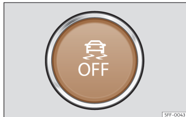
Fig. 172 In the lower part of the centre console: button to switch the ESC off/on
