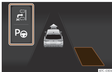
Fig. 174 On the instrument panel display: view of the parking assist system with reduced view.
