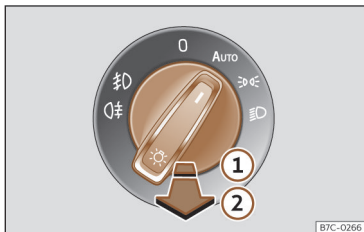
Fig. 88 Dash panel: lights control.
