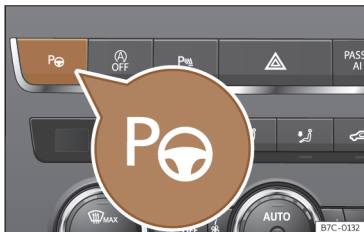
Fig. 173 In the upper part of the centre console: button to switch on the Park Assist system.
