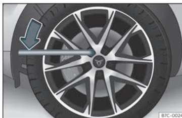
Fig. 34 Wheel change: loosen the wheel nuts.
