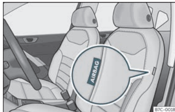
Fig. 19 Side airbag in driver's seat.
