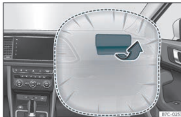
Fig. 14 Front passenger airbag located in dash panel.
