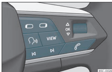
Fig. 62 Right side of the multifunction steering wheel: buttons for using the instrument cluster's menus and information displays (depending on versions).
