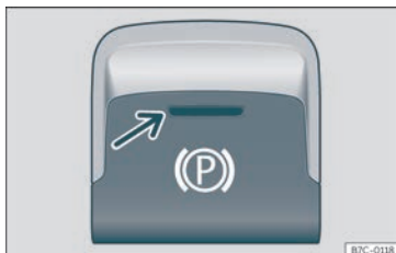
Fig. 175 In the lower part of the centre console: electronic parking brake button
