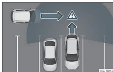
Fig. 174 Schematic representation of the rear cross traffic alert assistant: zone monitored around the vehicle while leaving a parking space.
