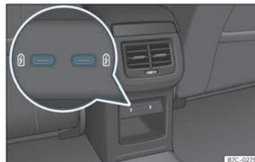
Fig. 138 Rear part of the centre console: USB connectors with power outlet function.
