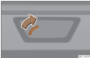
Fig. 87 Detail of the luggage compartment: emergency unlocking
