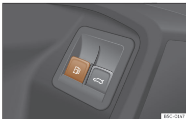
Fig. 201 Driver's door: tank flap release.
