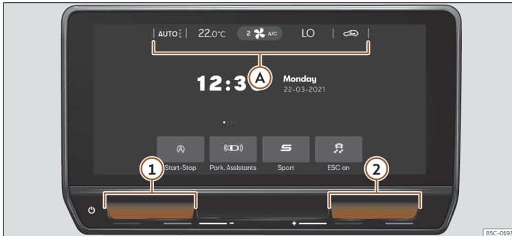
Fig. 129 Schematic representation: air conditioning functions
