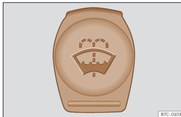
Fig. 216 In the engine compartment: window washer tank cap.
