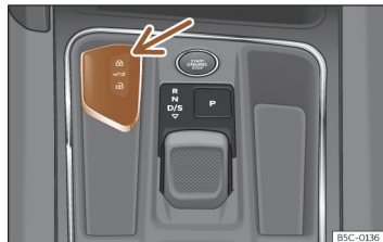
Fig. 71 Centre console: vehicle key socket.
