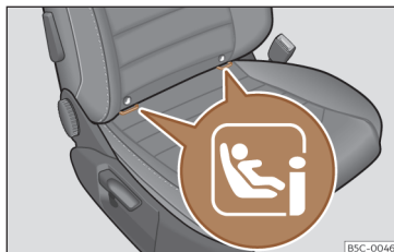
Fig. 28 Front passenger seat: ISOFIX/i-Size securing rings.
