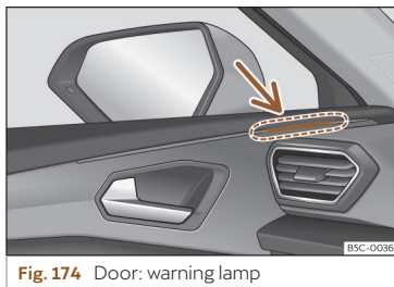
Fig. 174 Door: warning lamp
