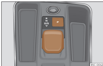
Fig. 145 In the centre console: selector lever.
