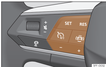
Fig. 155 On the multifunction steering wheel: buttons to operate the speed limiter.
