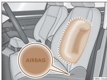
Fig. 21 Side airbag in driver's seat.
