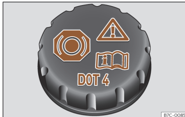
Fig. 215 Engine compartment: brake fluid reservoir cap.
