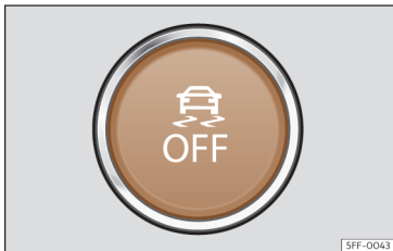
Fig. 177 In the lower part of the centre console: button to switch the ESC off/on
